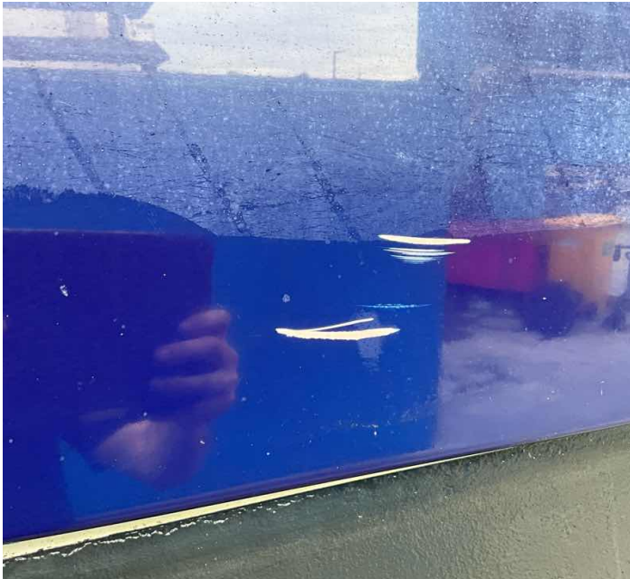
L17d. Various gouges to gelcoat on boat hull sides
