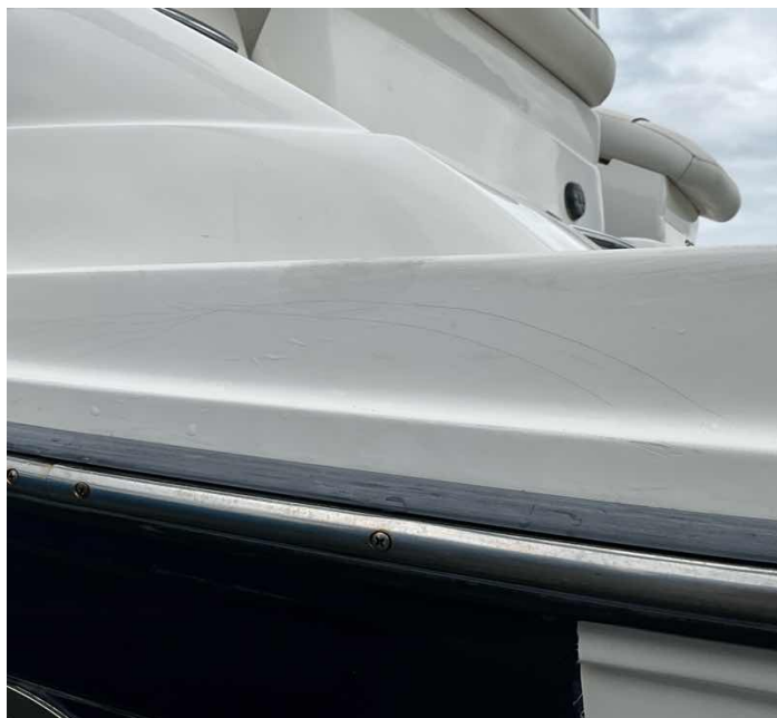
L18. Spider cracking to port side aft corner
