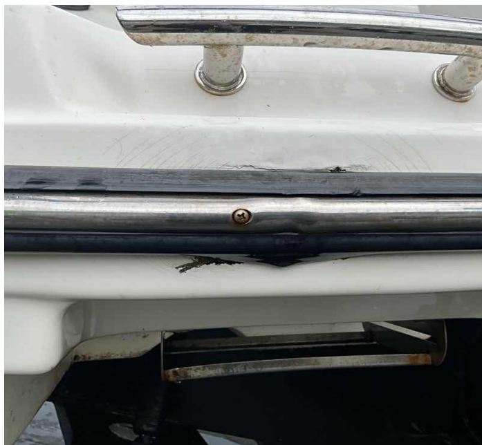
L21. Impact damage to port side aft corner of gunnel
