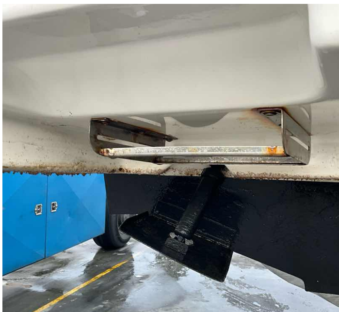
L19a. Swim platform ladder has been removed and replaced with aftermarket
