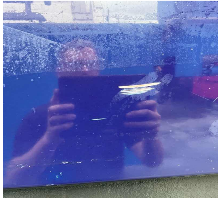
L17e. Various gouges to gelcoat on boat hull sides
