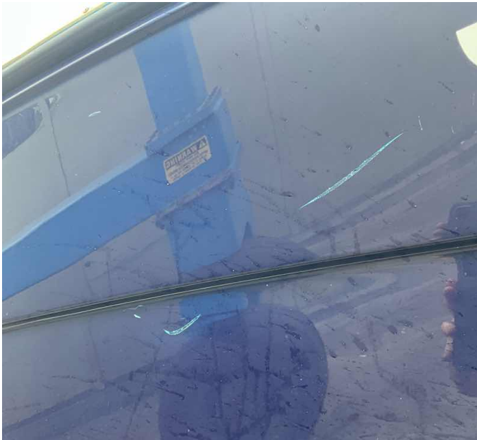
L17b. Various gouges to gelcoat on boat hull sides
