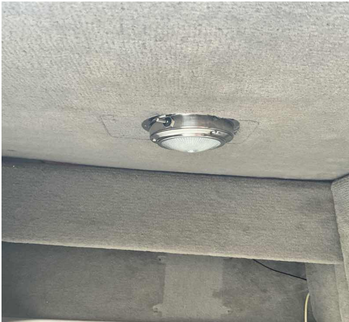
L6. Starboard side storage locker light out of order
