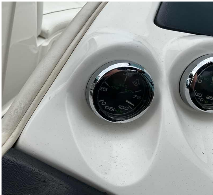
H1. Oil pressure sender appears faulty
