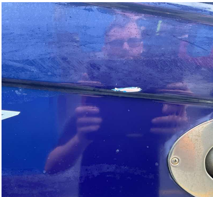
L17f. Various gouges to gelcoat on boat hull sides
