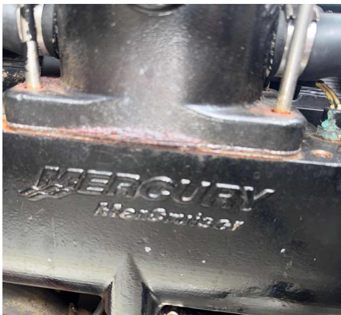
M3. Corrosion to exhaust manifold and riser gasket
