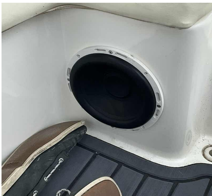
L12. Starboard rear speaker missing cover
