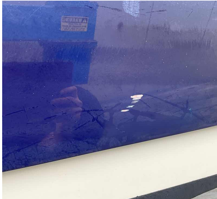
L17a. Various gouges to gelcoat on boat hull sides
