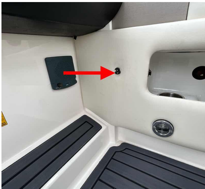
L10. VHF transmitter missing
